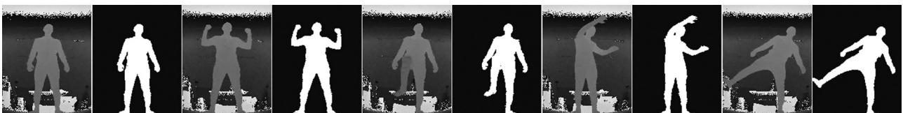
Fig. 5. Results of foreground segmentation in the Stanford dataset: pairs of original and foreground images.
